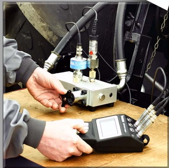
Faultfinding on a tractor with the HPM460
