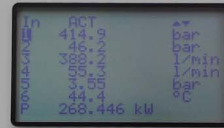
Screen shot of HPM460 showing 6 values on screen at once and calculated power.
