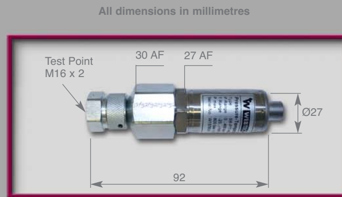
Note: M16 x 2 adaptor also available in two piece 316 SS version
